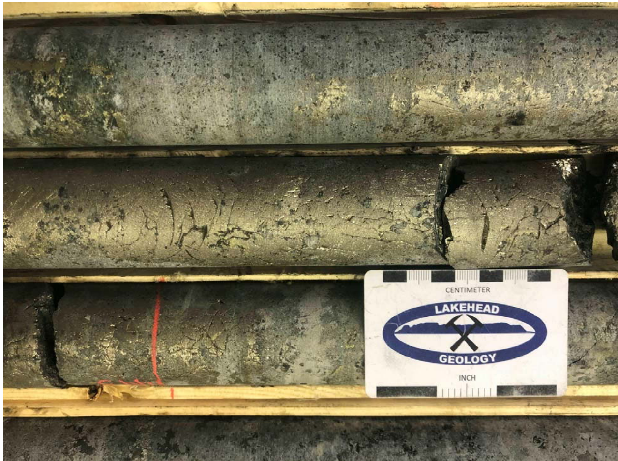
Figure 4: Marathon Project – Photograph of massive sulphides from Hole M-20-543 interval 433-449 m
